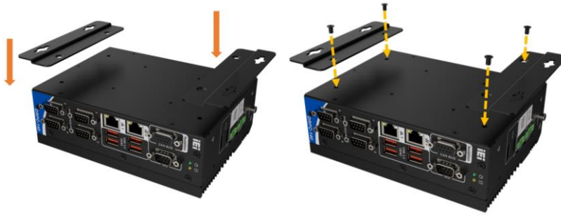
Figure 3-13: Mounting Bracket Retention Screw
