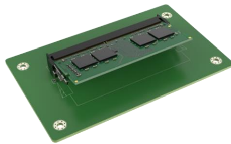
Figure 3-3: Insert the Memory Module
